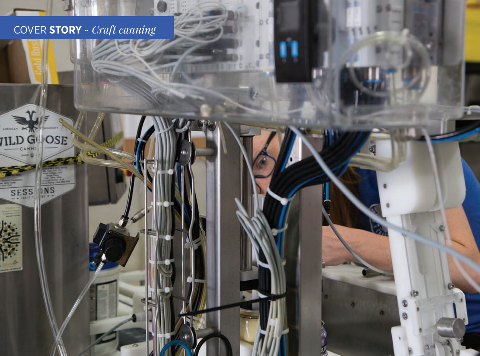
Sessions Craft Canning lead canning line operator Ellen Dannys performs a regularly scheduled maintenance overhaul on one of its mobile filling and capping lines manufactured by Wild Goose Canning at the Sessions HQ to maintain top-notch efficiency when on the road at a craft brewery, cidery or beverage producing facility.
